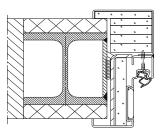
enclosing frame corner frame with supplementary frame
