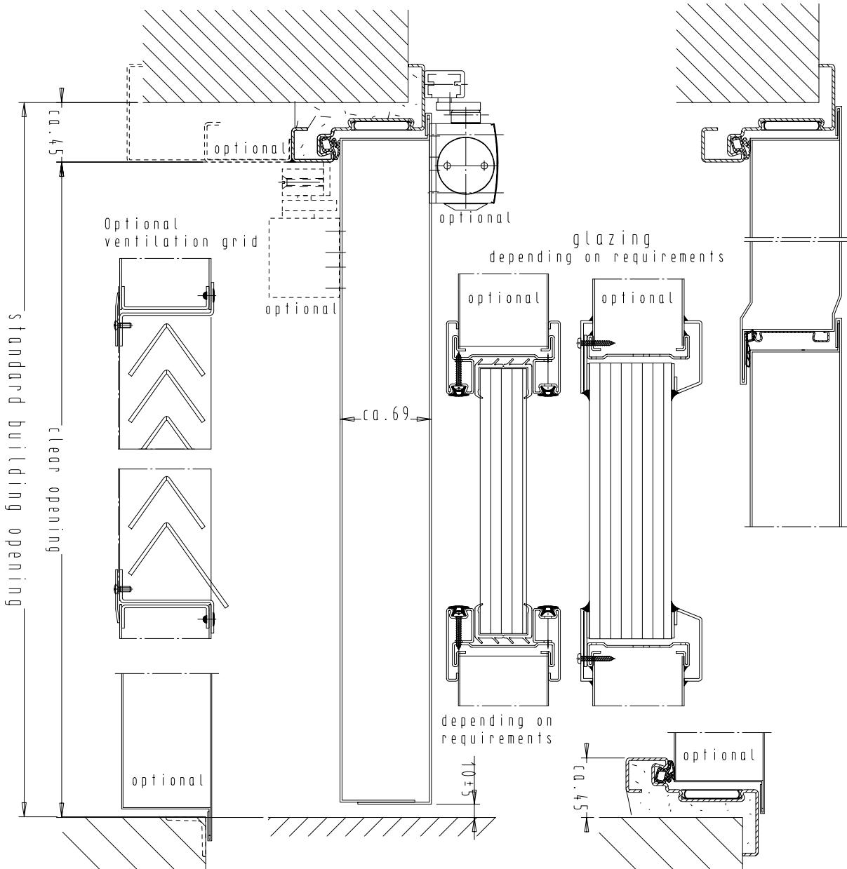
Optical ventilation cross-section 70%
